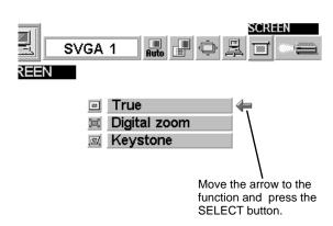
NOTE: The True and the Digital Zoom cannot be operated when "RGB," "HDTV1035i" or "HDTV1080i" is selected on the SYSTEM MENU (P22 and 23).
